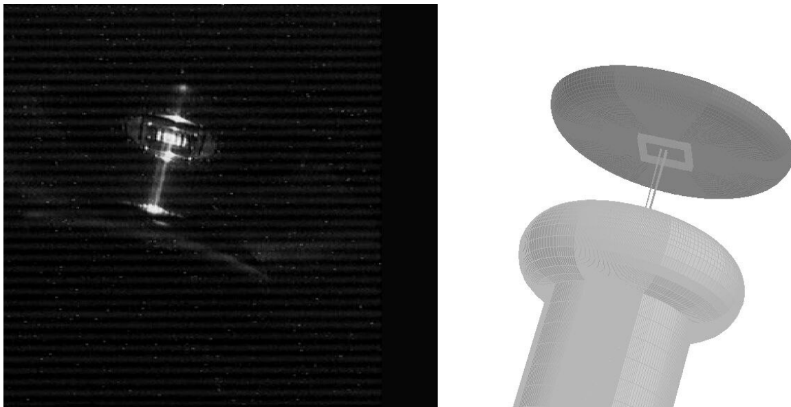
Figure 7. Post-acceleration of three beamlets in ITER-like SINGAP. To the left a photo from the beam taken from above at an oblique angle. To the right a SCALA simulation of shot 7545 viewed from a similar direction. The two beamlets on the right appear as one bright beamlet because the line of sight passes through both of them.
