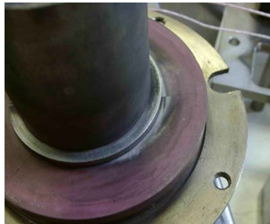
Fig.7. Metal deposition to cathode-anode insulator
