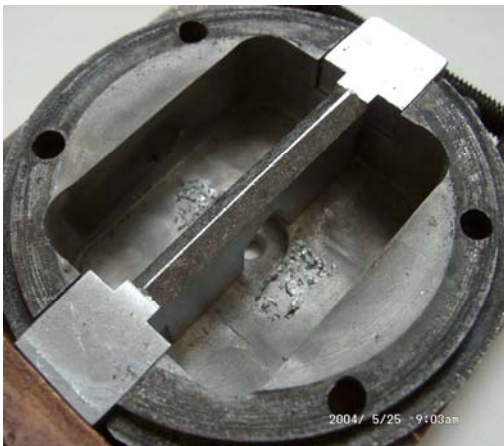
Fig.6. Molybdenum flakes deposition on the anode (after one month of experiments)
